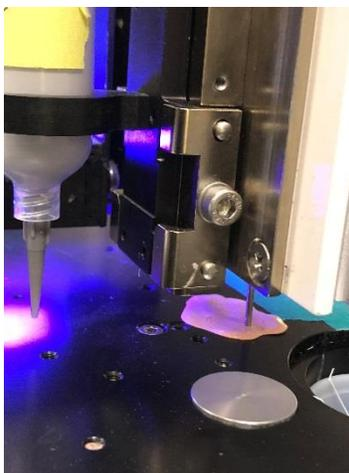
10. On the “Align camera on probe mark and press [Teach]” window, move the dispenser stage until the cursor on the camera screen lies in the center of the mark on the silly putty made by the probe, Then press “Teach”.
